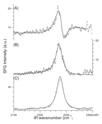
**Figure 4.** SFG spectra of PAN in PPP polarization at the (A) PAN/air, (B) PAN/water, and (C) PAN/heptane interfaces collected from 2150 to 2300 cm<sup>-1</sup>. The solid lines are the fits using a Lorenztian equation.
