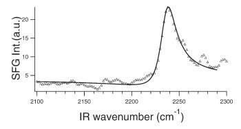
**Figure 2.** SFG spectrum of PAN in PPP polarization in the CN region at the sapphire/PAN interface after the PAN film is annealed at 90 °C for 8 h. The solid line is a fit using a Lorenztian equation.
