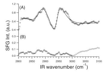
**Figure 3.** (A) SFG spectrum of PAN in PPP polarization at the heat-treated sapphire/PAN interface. The PAN films were annealed at 90 °C for 8 h and 120 °C for 4 h after spin-coating on a heat-treated sapphire prism (750 °C for 36 h). (B) SFG spectrum of PAN in PPP polarization after annealing at 90 °C for 8 h and 120 °C for 4 h at the sapphire/PAN interface. Both these spectra are shown in the CH stretching region.
