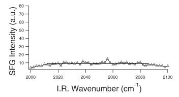
**Figure 5.** SFG spectrum in PPP polarization for the PAN/water interfaces collected between 2000 and 2100 cm<sup>-1</sup>. This spectrum was collected using the SFG laser system at Akron that uses a 800 nm visible laser (1 kHz and pulse width of 1–2 ps) and mixes with tunable IR generated using an OPA (1 kHz and pulse width of 1–2 ps).
